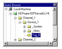
6. Close the browser window by clicking in the **Close** box in the upper-right corner. The new input path **Channel\_1. Device\_1.Tag\_R** will appear in the **Item ID** field.
